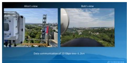
This kind of equipment is smaller in size and weight and the system is more secure because of point-to-point connection. This solution is immune to electromagnetic interference.
